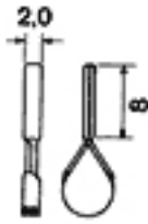
Mini Vessel Clip ZI-04-102-08 jaw 8,0 x 2,0 mmclosing pressure 100 gr.
