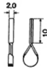
Mini Vessel Clip ZI-04-102-10 jaw 10,0 x 2,0 mmclosing pressure 125 gr.
